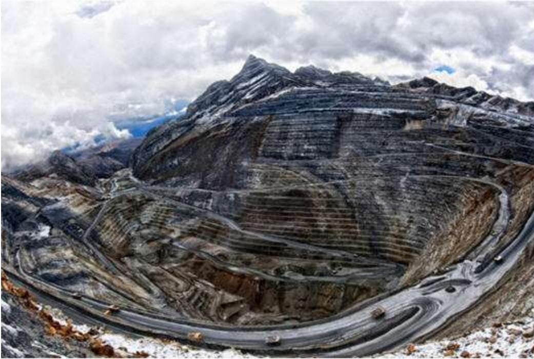
**Antamina is a skarn deposit with associated regional porphyry mineralization**
